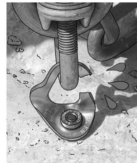
ancrage Long Life Petzl rupture plaquette 2508 daN.
